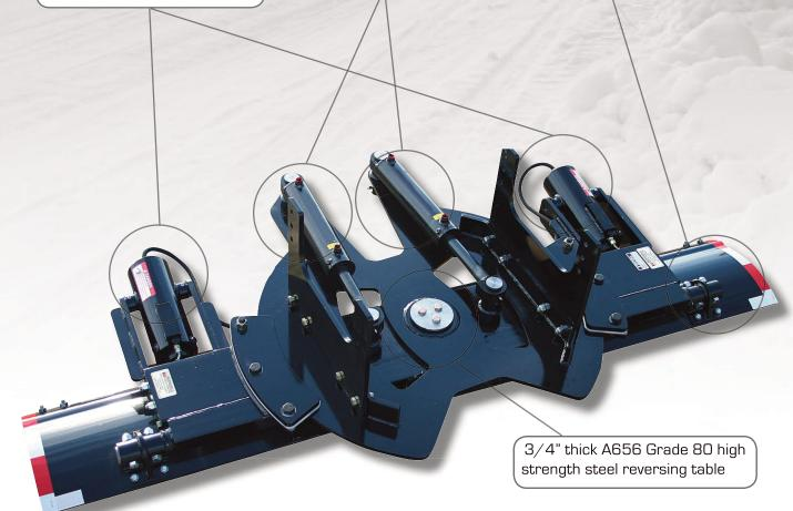
The Bonnell Power Reversing Under Body Scraper is available in 10', 11' or 12' lengths, and is power reversable up to 45 degrees left or right. The Scraper has a 1" thick .40/.50 carbon steel moldboard with a 20" tall, smooth formed inside radius, offset to accommodate the cutting edge.
