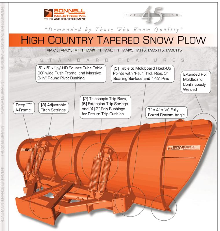
Bonnell High Country Tapered Snow Plows are designed for removing snow at high-speeds in rural areas and interstate highways. The standard extended roll moldboard is designed to move the snow to the discharge end of the plow more efficiently. This prevents the snow from blowing over the top of the plow. This plow produces the same results when plowing to the left or to the right.
